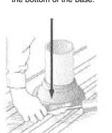
Step 4 Mold the flexible base to the panel contours.
